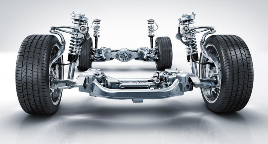
MAGIC BODY CONTROL detects bad road surfaces in advance and reacts accordingly. The active damping system of the suspension works with a road surface scan to achieve this
